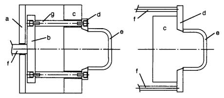
Figure 4.9 (*Left*) Section through stripper ring mold: (a) mounting plate, (b) ejector plate, (c) core plate, (d) stripper ring, (e) molded product, (f) machine ejector, (g) connecting sleeve. (*Right*) Section through stripper plate mold: (c) core and mounting plate, (d) stripper plate, (e) molded product, (f) machine ejectors.
