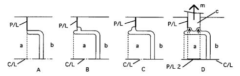
Figure 4.4 Schematic illustrations of location of parting lines (P/L) (only one half of mold shown): (a) core, (b) cavity. (A) Simplest case: P/L at right angles to axis of mold. (B and C) Product with rim but still simple. P/L can be either as in (B) or in (C). (D) Simple product but with rim and projection. Cavity is split, creating an additional P/L 2.
