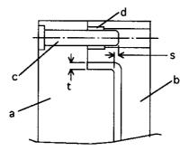
Figure 4.11 Typical mold with leader pin and bushing alignment: (a) core plate, (b) cavity plate, (c) leader pin, (d) leader pin bushing, (s) safety distance of pin above core, (t) wall thickness of plastic product at parting line.
