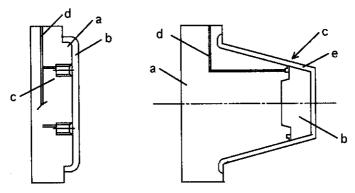
Figure 4.10 Air ejection alone. (*Left*) (a) core and mounting plate, (b) molded product, (c) air valves, (d) pressure air supply. (*Right*) (a) core and mounting plate, (b) core tip, (c) circular air gap, (d) pressure air supply, (e) molded product.
