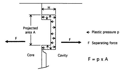
Figure 4.6 Portion of a schematic mold, showing a cavity filled with plastic under pressure acting in all directions.
