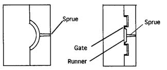
Figure 4.5 Illustration of schematic mold, showing cold sprue (left) and cold runner (right).
